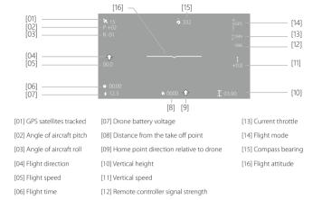
⚠ If [04] and [09] both point in the same direction, the drone is flying towards to remote controller/home point.
